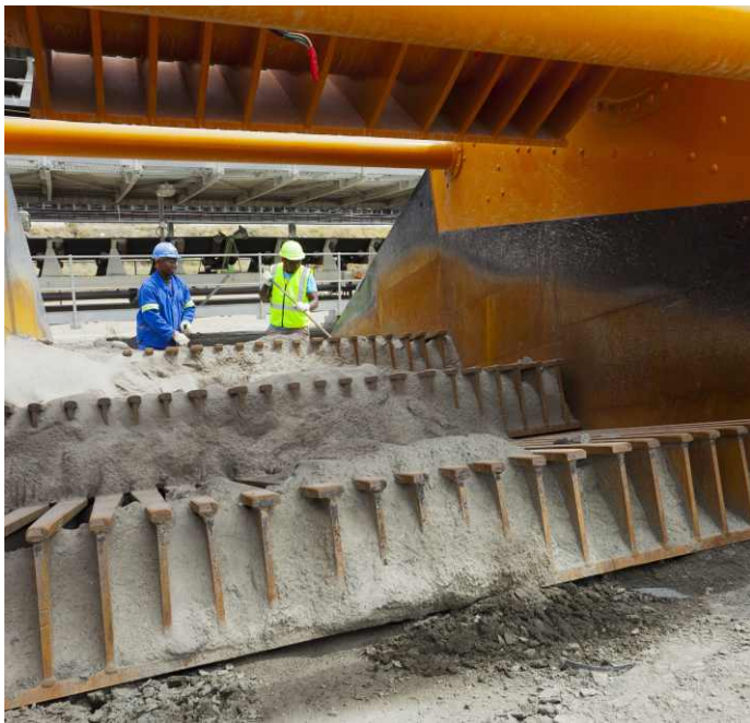
Checking a grizzly (left) and maintaining the spare grizzly unit (right) that enables quick change so there is minimal down time when the unit needs maintenance.
