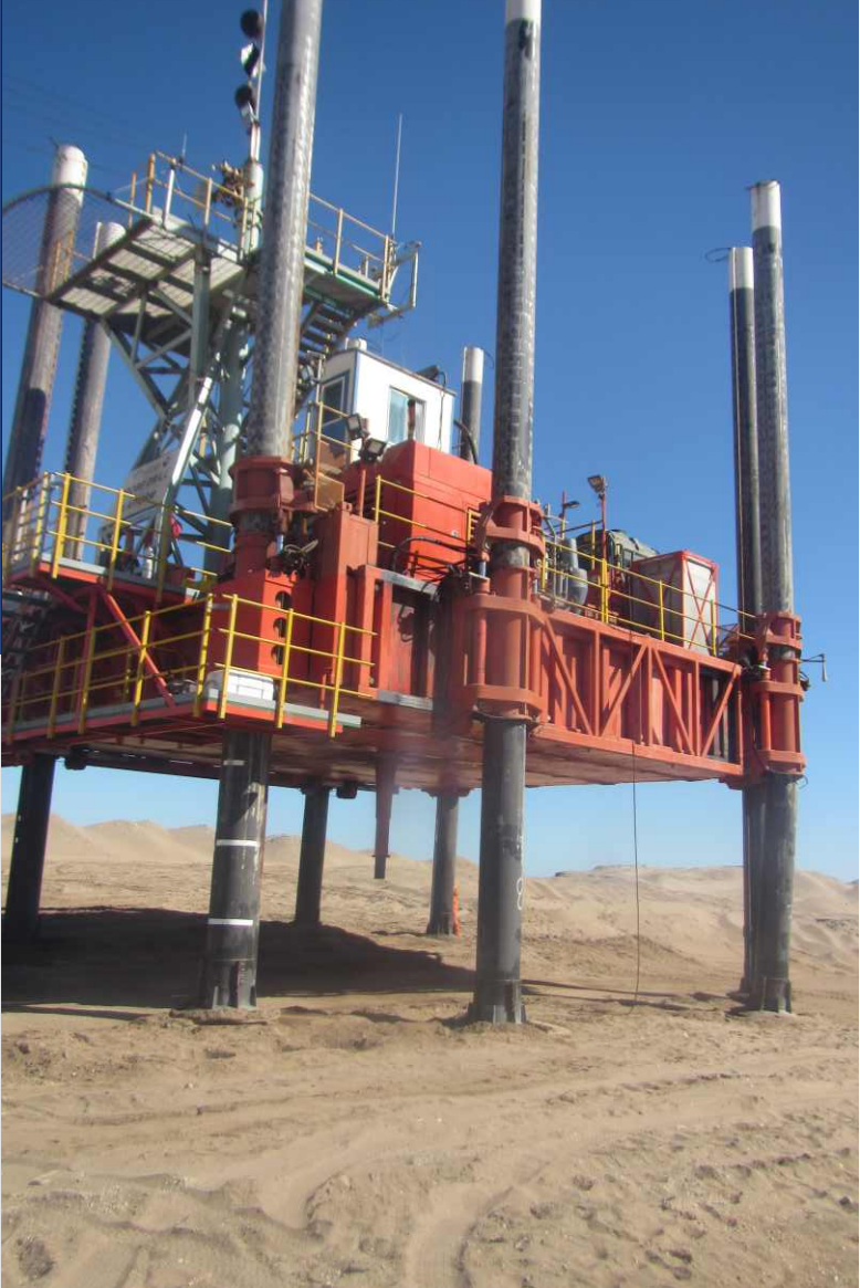
The probe drill platform (PDP) at an inshore diamond mining project in Namibia
