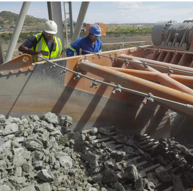
Checking a grizzly (left) and maintaining the spare grizzly unit (right) that enables quick change so there is minimal down time when the unit needs maintenance.
