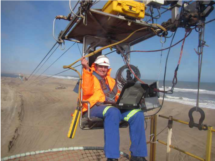
Jaco Pretorius, senior machinery inspector for Field Services, conducting a magnetic rope test for Namdeb in Namibia
